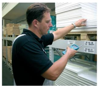
The Nordic ID RF601 is part of a unique wireless data collection system. The system consists of radio handsets that are used to communicate with the host system via base stations using an efficient communication protocol. The host system
