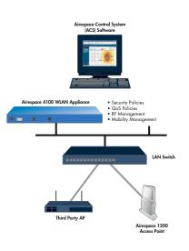
The Airespace 4100 comes in two models – the Airespace 4101, which provides a single Gigabit Ethernet uplink for high speed connectivity to existing wire-line devices, and the Airespace 4102, which provides two Gigabit Ethernet interfaces for redundancy.
